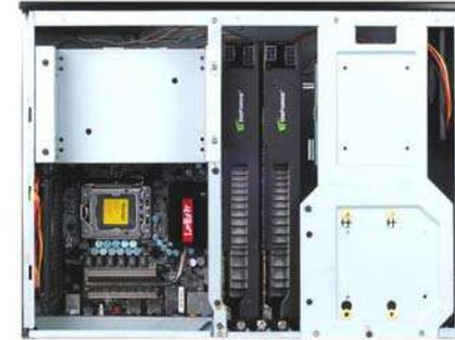
Although the chassis measures only 325mm deep, it can support powerful graphics cards for high end configurations.
