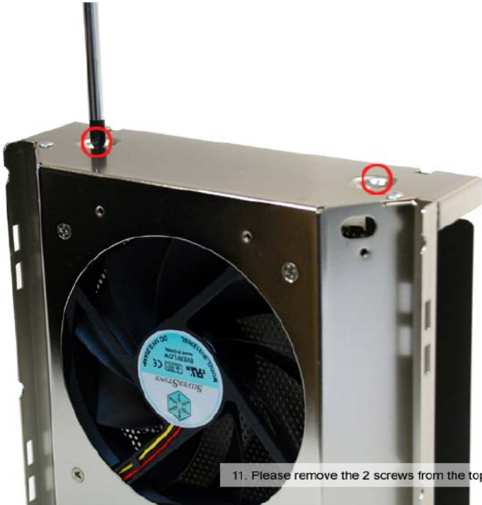
10. Remove the fan bracket from the case
