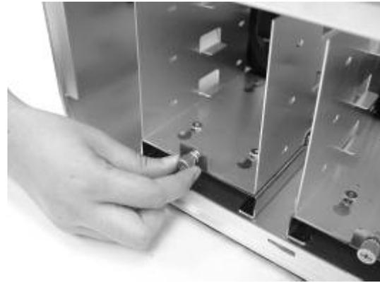
14. Loosen the thumb screw holding the 3.5" drive cage
