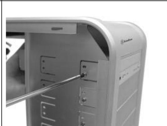
12. Align the drive or device to appropriate positions and secure with PW-M3\*6 screws as shown
