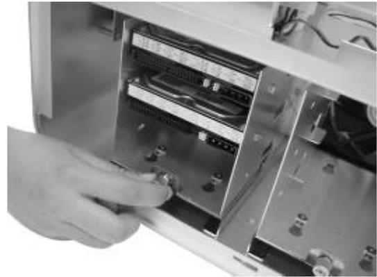
20. Secure drive cages by tightening the thumb screws
