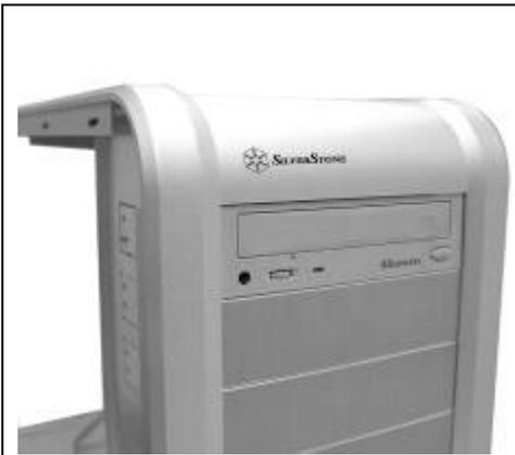
13. An installed optical drive shown
