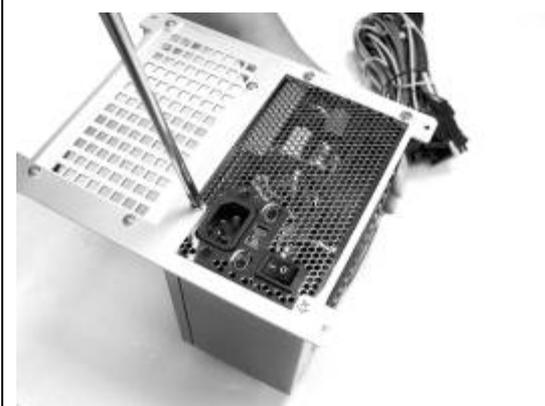
23. Align the power supply to the PSU plate and secure with HW#6-32\*6 screws
