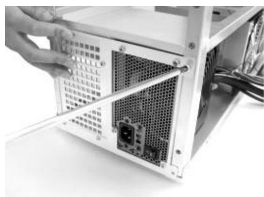
24. Install both PSU plate and the power supply back into the case
