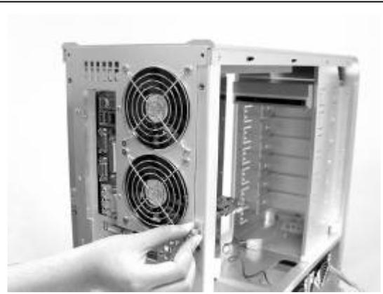
26. Secure motherboard tray with all six thumb screws and proceed to connect all cables and wires to complete system install
