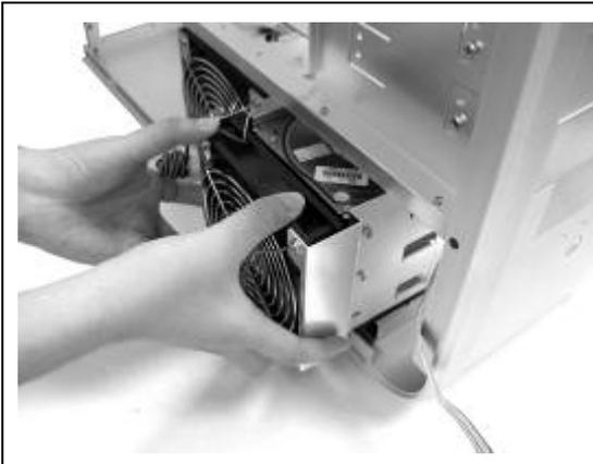
19. Insert 3.5" drive cage back into the case
