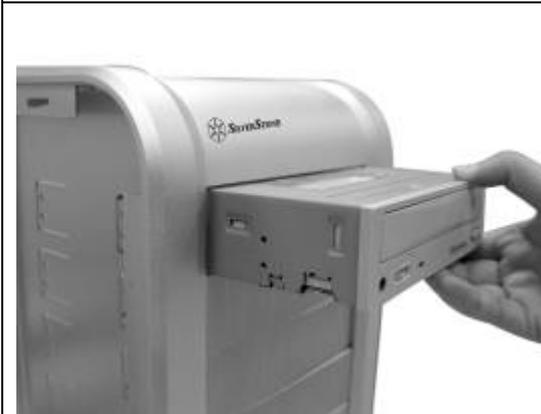
11. Insert optical drive or other 5.25" device into the drive bay
