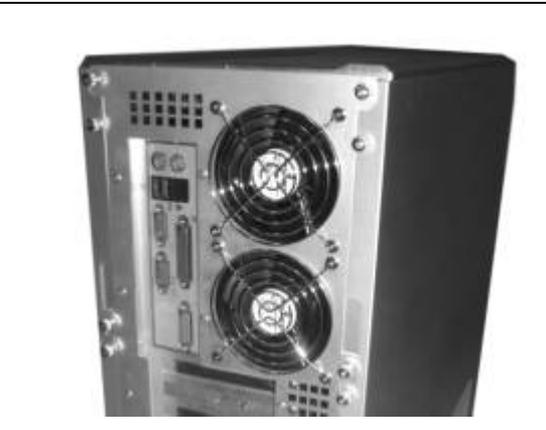
28. Secure both side panels with thumb screws
