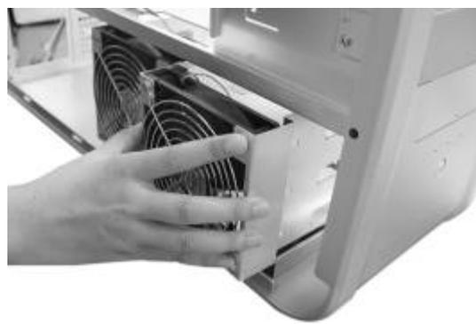
15. Slide drive cage to one side as shown to remove it
