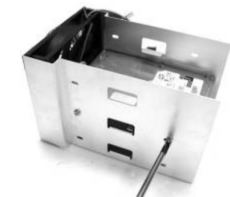
17. Insert hard drive into the drive cage and secure with HW#6-32\*6 screws
