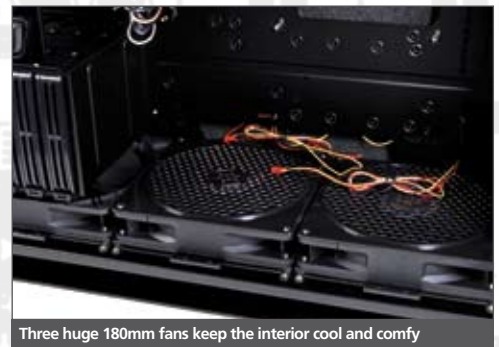
Three huge 180mm fans keep the interior cool and comfy
