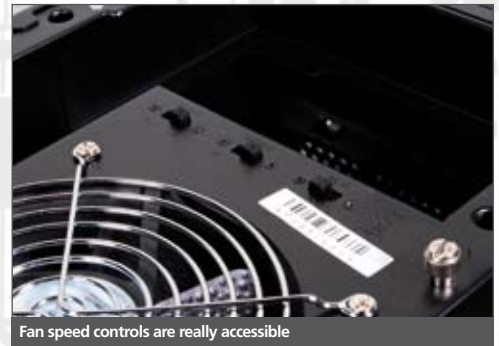
Fan speed controls are really accessible
